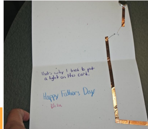
Electric art can be two or three-dimensional. All electric art needs to have switches. Here is one example. When the card is closed, the copper tape touches the battery and completes the circuit.
