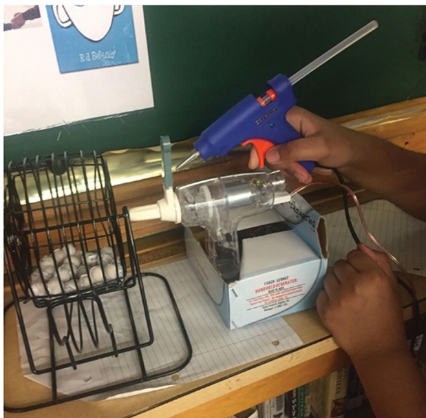
Figure 8. Light-up bingo cage version 2: Gluing the hand crank to the Bingo Cage.
